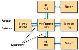
HyperTransport is based on dual point-topoint unidirectional links consisting of datapaths, control signals, and clock signals. Each datapath can be from 2 to 32 bits wide. Commands, addresses, and data share the datapath. A link consists of the datapath, a control signal, and one or more clock signals. A complete HyperTransport-based system consists of a processor with a HyperTransport port, an input link and an output link, and any I/O channels connected to the HyperTransport bus.
