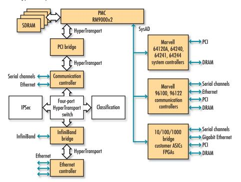
200 to 800 MHz. It delivers more bandwidth than other available alternatives, uses lowlatency responses, minimizes pin counts, ensures compatibility with legacy PC buses and transparency to operating systems, extends to new SNA buses, and causes minimal impact on peripheral drivers. These extensive capabilities position it as the most comprehensive I/O bus solution for the next generation of embedded systems.
