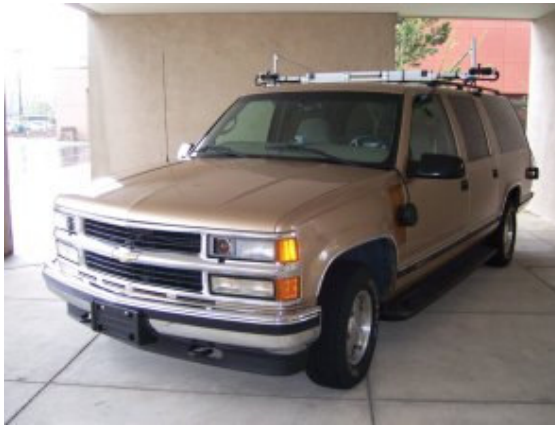
The initial development stage for the heavy truck IVBSS platform utilised a Chevy Suburban pulling a trailer to simulate the size and scope of a tractor-trailer rig
